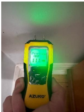
Pic29 & 30 example moisture readings
